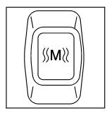
If your vehicle has this feature, the switch is located on the outboard side of the front seats behind the lumbar switch. Press the switch to turn the massaging lumbar feature on. The ignition must be on.
